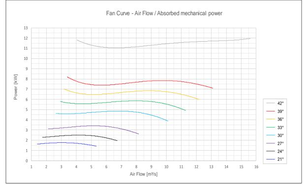
Impeller size 1000 mm - (1480 rpm)
