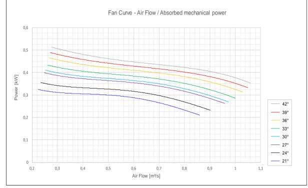
Impeller size 400 mm - (2900 rpm)
