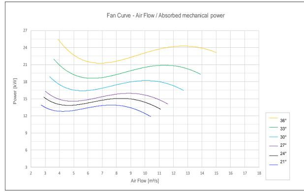
Impeller size 630 mm - (1480 rpm)
