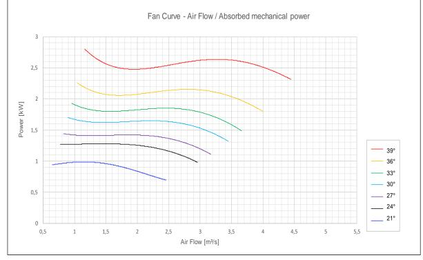
Impeller size 630 mm - (2900 rpm)
