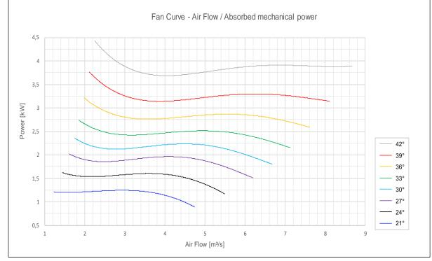
Impeller size 800 mm - (1480 rpm)
