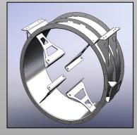
The motor support wings are designed to ensure the necessary rigidity to the system and in the same time ensuring high aerodynamic efficiency.
